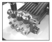
18. Replace plug with o-ring (48, & 48A) and tighten to 160 ft.-lbs.
